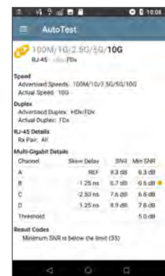
Cabling SNR measurement validates Multi-Gig links
